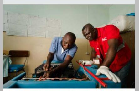
Coca-Cola Lead Cooler Technician, Maxwell Ayisi (right), and Ghana Health Service Refrigeration Technician, Livingstone Modey (left), repairing a dual gas/electric cooler used to store vaccines at a clinic in Peki Dzake in the Volta Region of Ghana.
